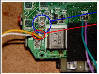
After this mod I put the fm deviation pot VR401 to the maximum (turn left). Mine has peaks now to about 2,5 kHz deviation (original peaks were only 1,5 kHz!).
