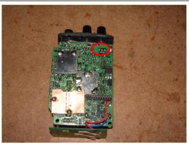
Solder a 1n - 1,5n (not critical) capacitor between the both ends of the VOL pot. That means parallel to the vol pot.
