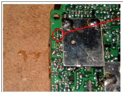
Replace C26 with a higher value to give the tx smeter a better average readout.
