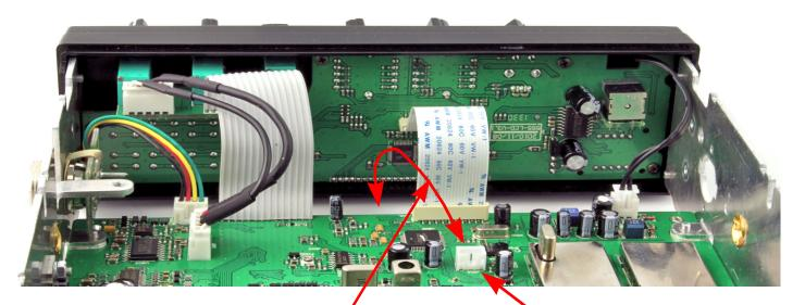
Plug the end of the programming cable with the white connector in here and run cable to front and on the other side of the main circuit board and out notch in chassis at the rear of radio. Used the supplied plastic cap to protect the connector.
